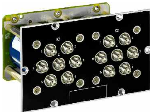
Figure 7 Module R&S OSP-B102
